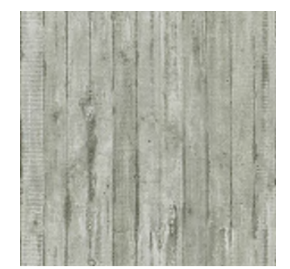
FORMED BOARD CONCRETE
