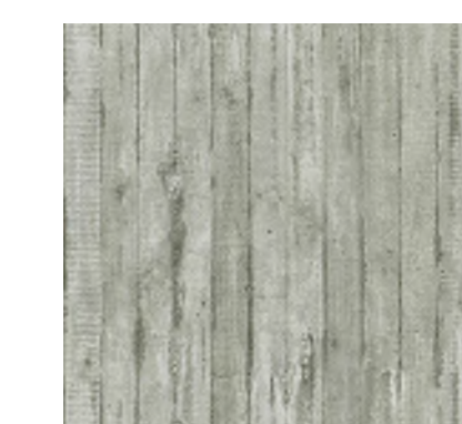
FORMED BOARD CONCRETE
