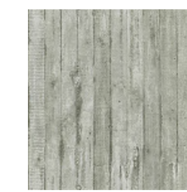
FORMED BOARD CONCRETE
