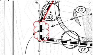
Response: Opening in silt fence is shown on plans and check dam has been added to low point as shown in markup.
