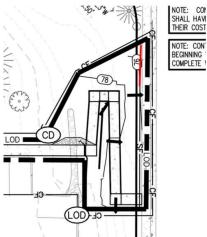
Response: Acknowledged – silt fence limits extended to limits of disturbance. Linework on plan adjusted as per above-mentioned comment. Thank you for your review.
