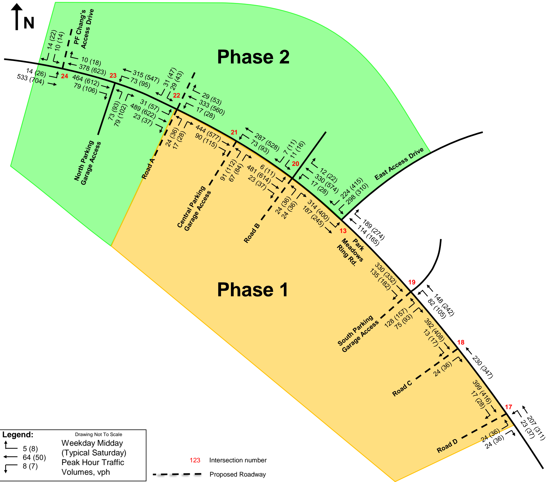
2045 (Long-Range – Phase 1 & 2 Buildout) Total Midday Peak Hour and Typical Saturday Peak Hour Traffic Volumes (Internal Intersections)
