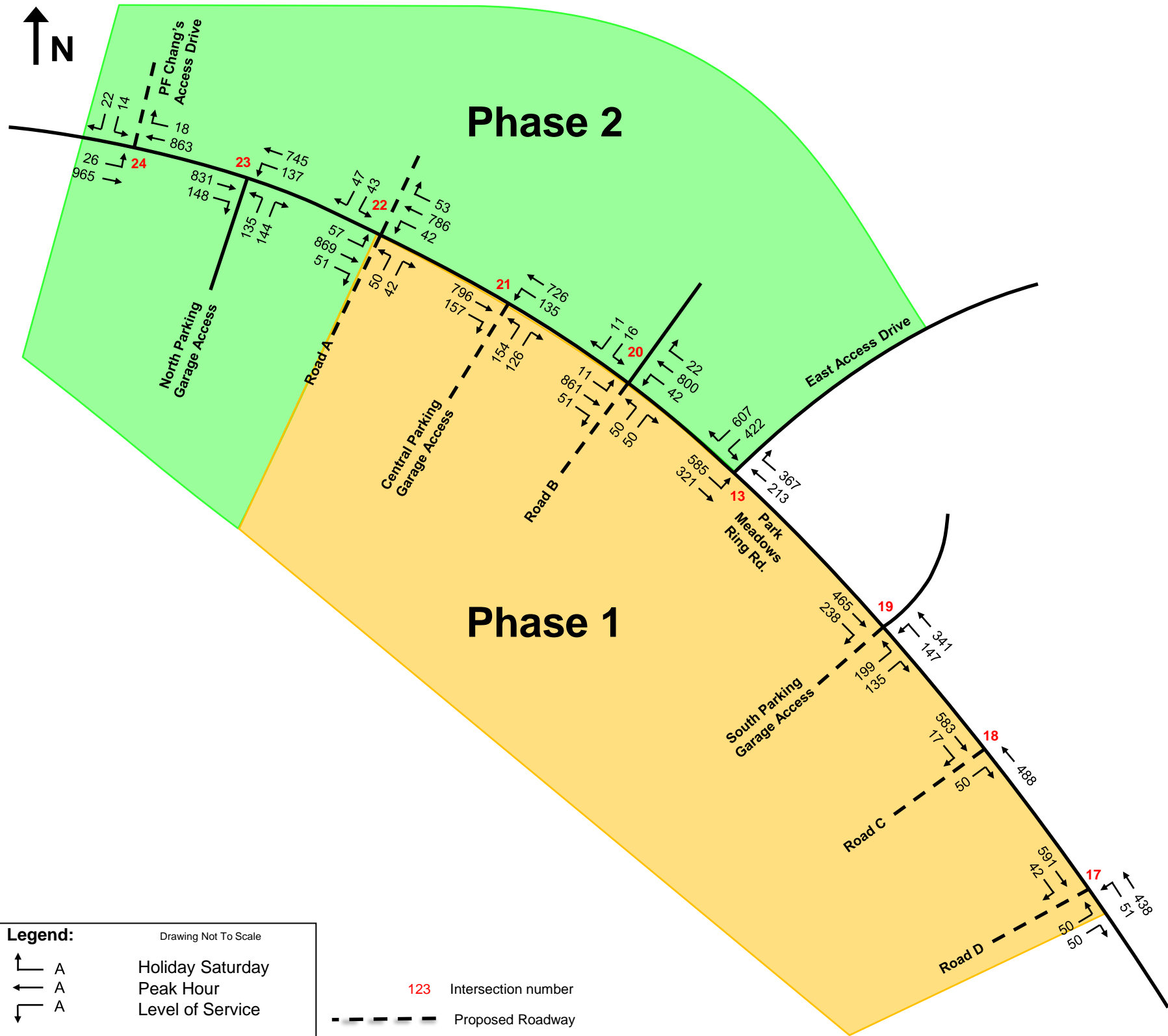
2045 (Long-Range – Phase 1 & 2 Buildout) Total Holiday Saturday Peak Hour Traffic Volumes (Internal Intersections)
