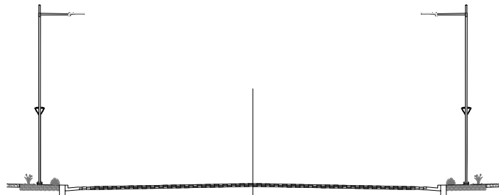
STRATEGY 3: STREET LIGHTING AT INTERSECTIONS WITH NON-CONTINUOUS PEDESTRIAN LIGHTING *STREET LIGHTING ALTERNATING 300' SPACING
