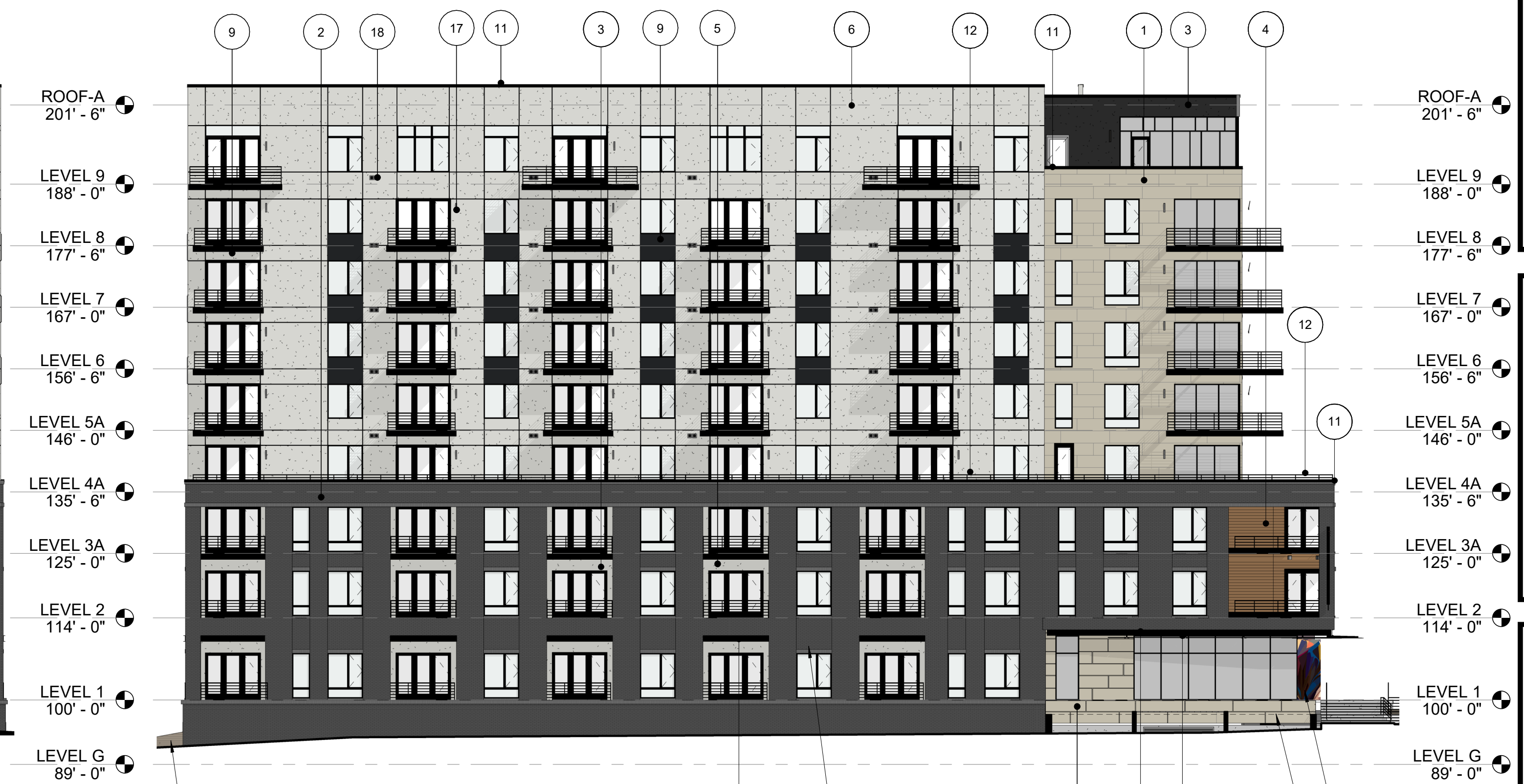
1 SIP NORTH ELEVATION 1/16" = 1'-0"
