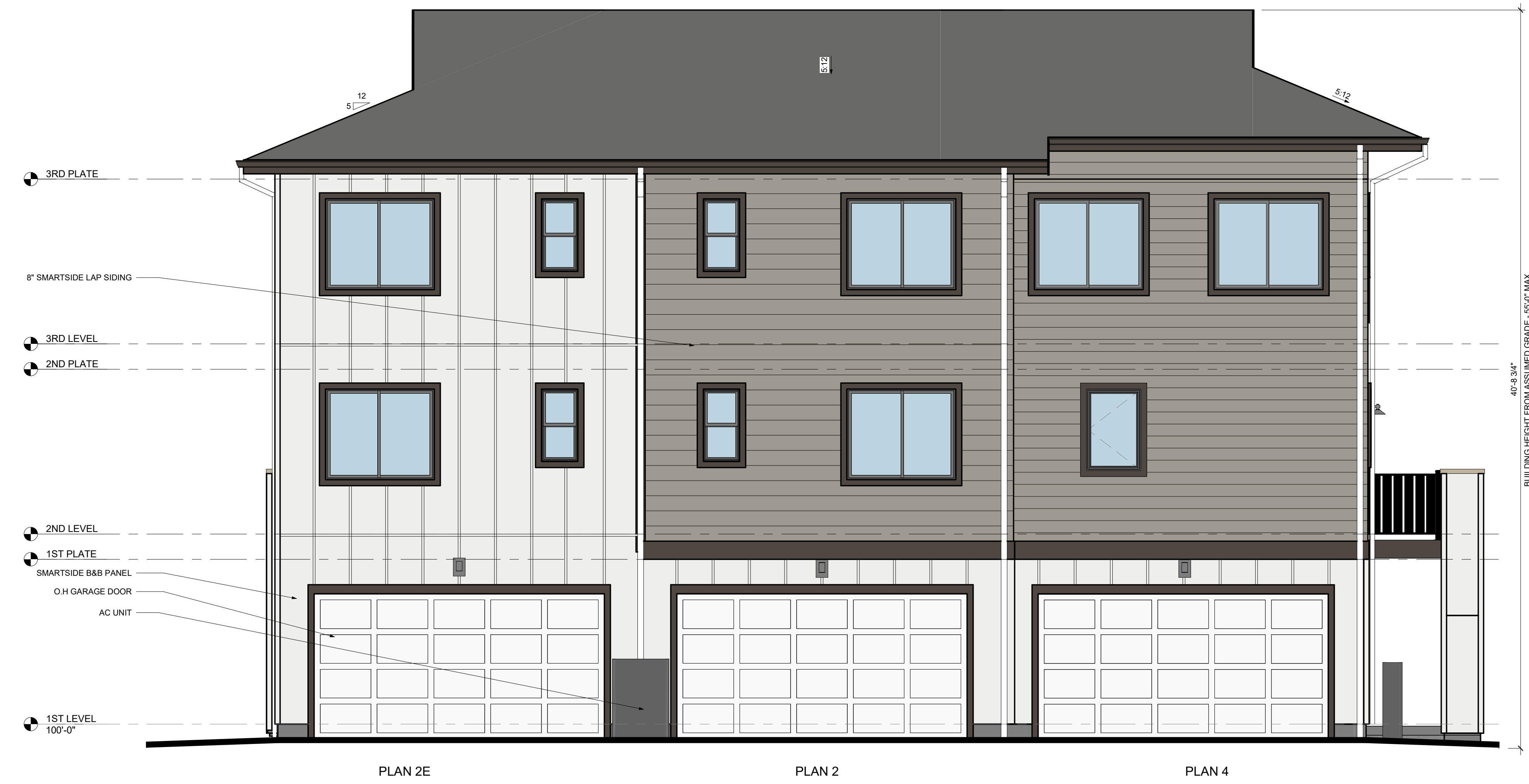
1 3B - REAR ELEVATION - CONTEMPORARY - SCHEME 2 1/4" = 1'-0"
