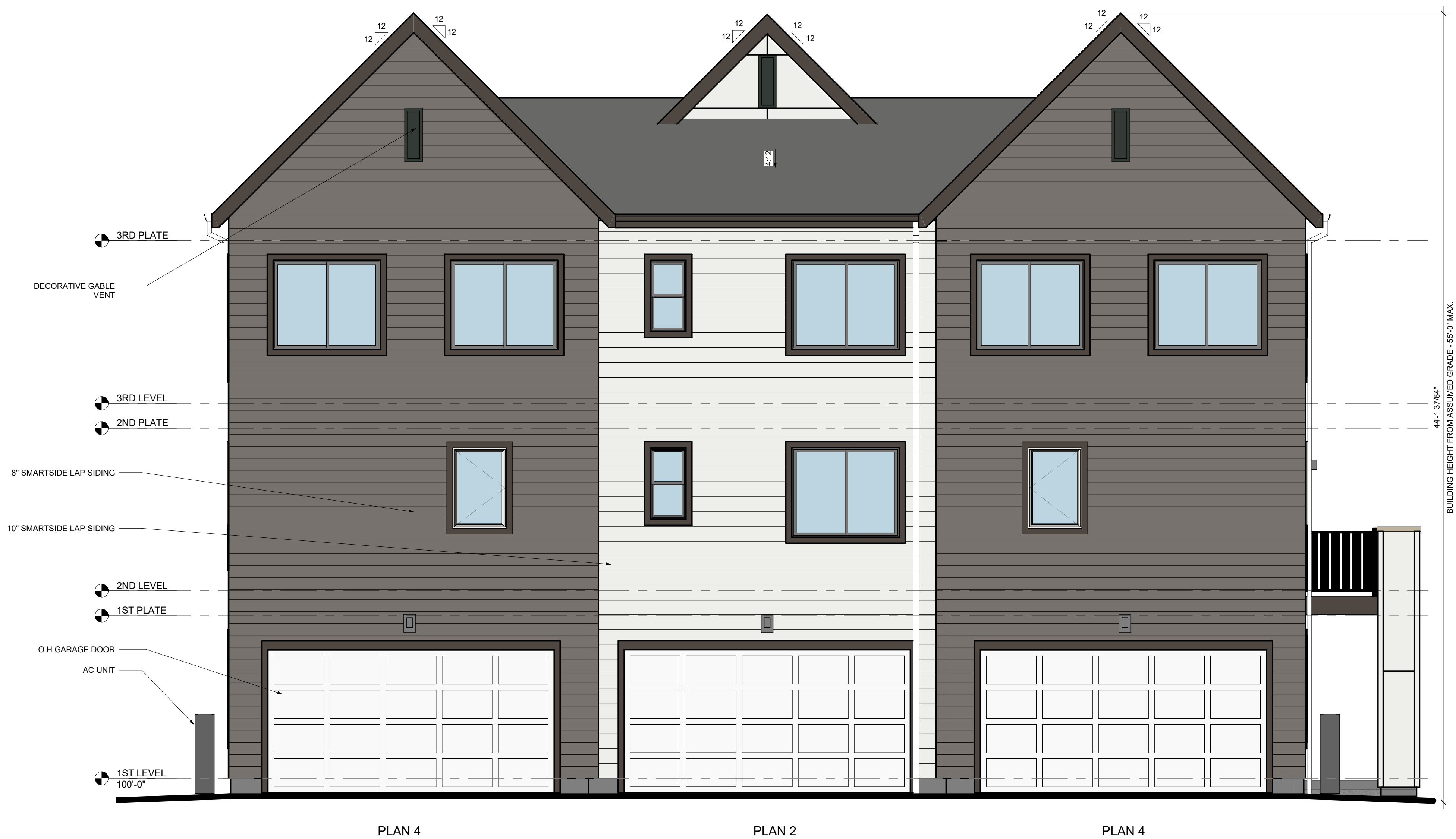
1 3A - REAR ELEVATION - TRANSITIONAL - SCHEME 1 1/4" = 1'-0"
