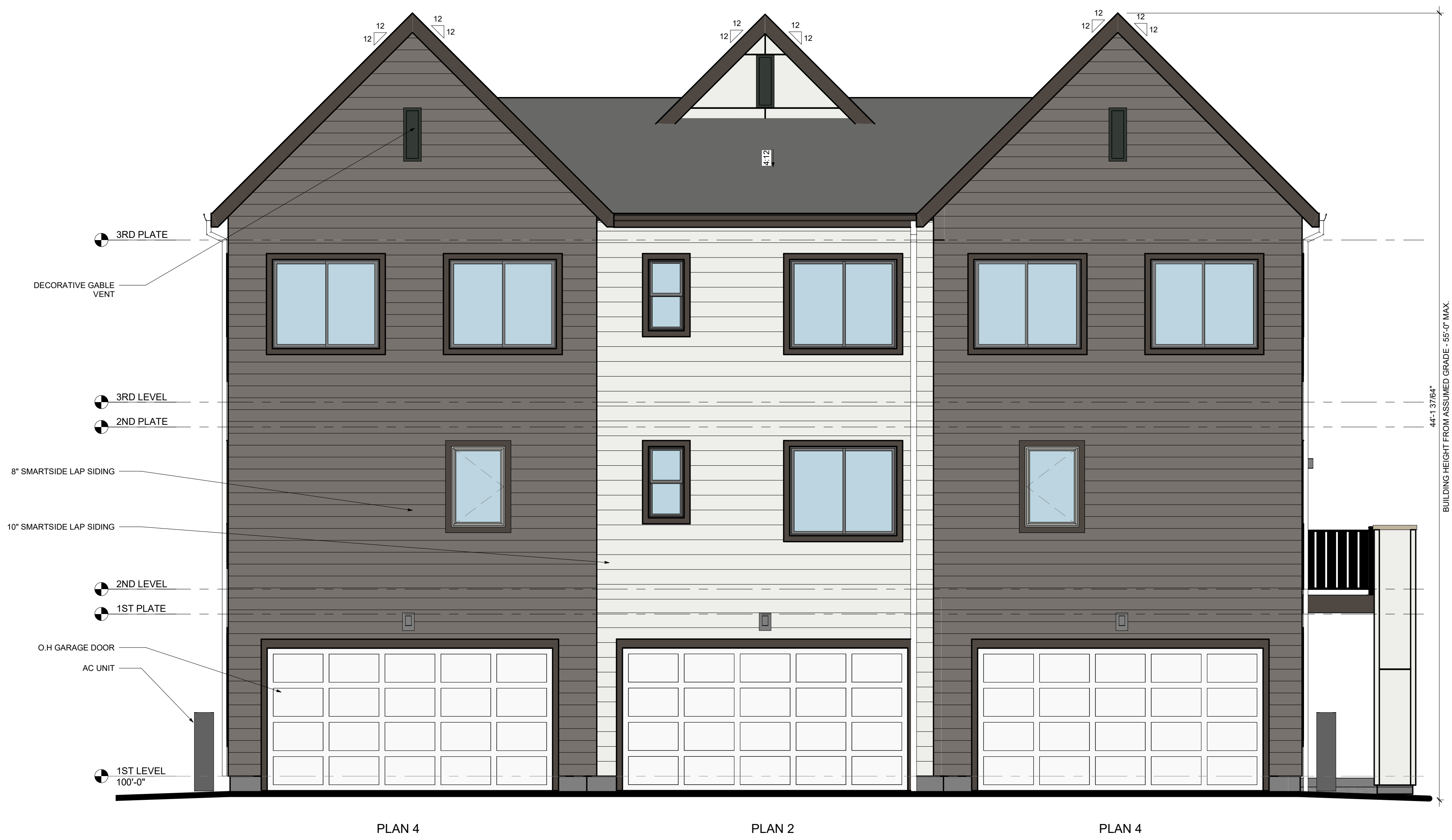
1 3A - REAR ELEVATION - TRANSITIONAL - SCHEME 1 1/4" = 1'-0"
