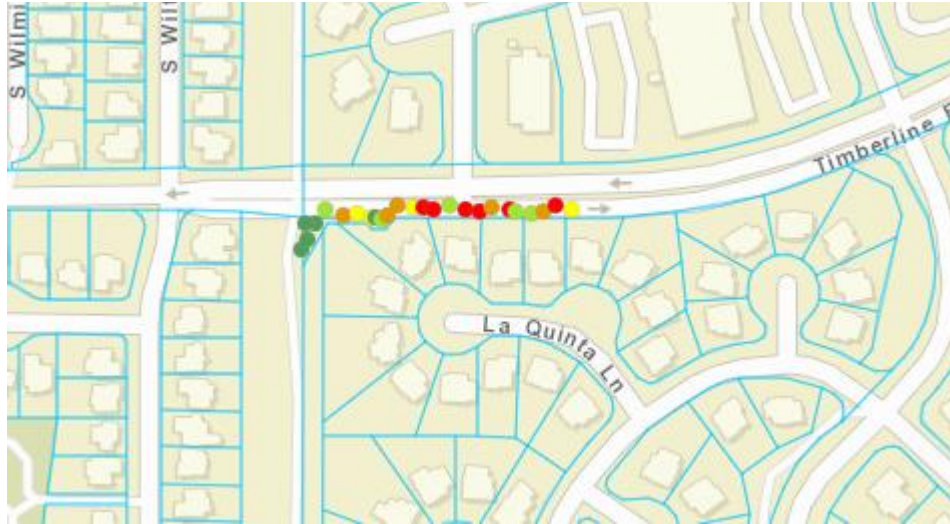
Figure 66. Screenshot from GIS software showing a sample of grade data displayed at the actual panel locations on a street map.
