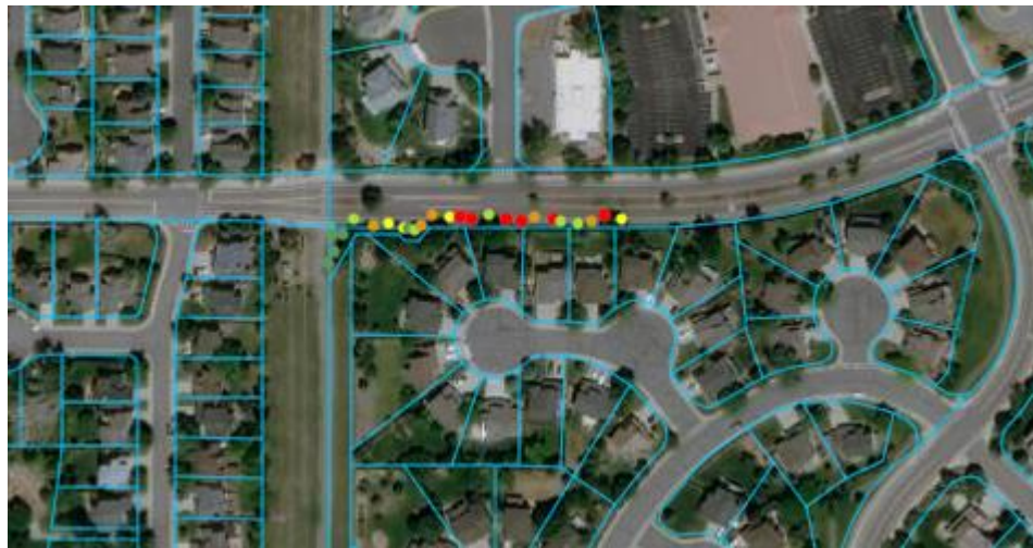
Figure 65. Screenshot from GIS software showing a sample of grade data displayed at the actual panel locations on a satellite view.
