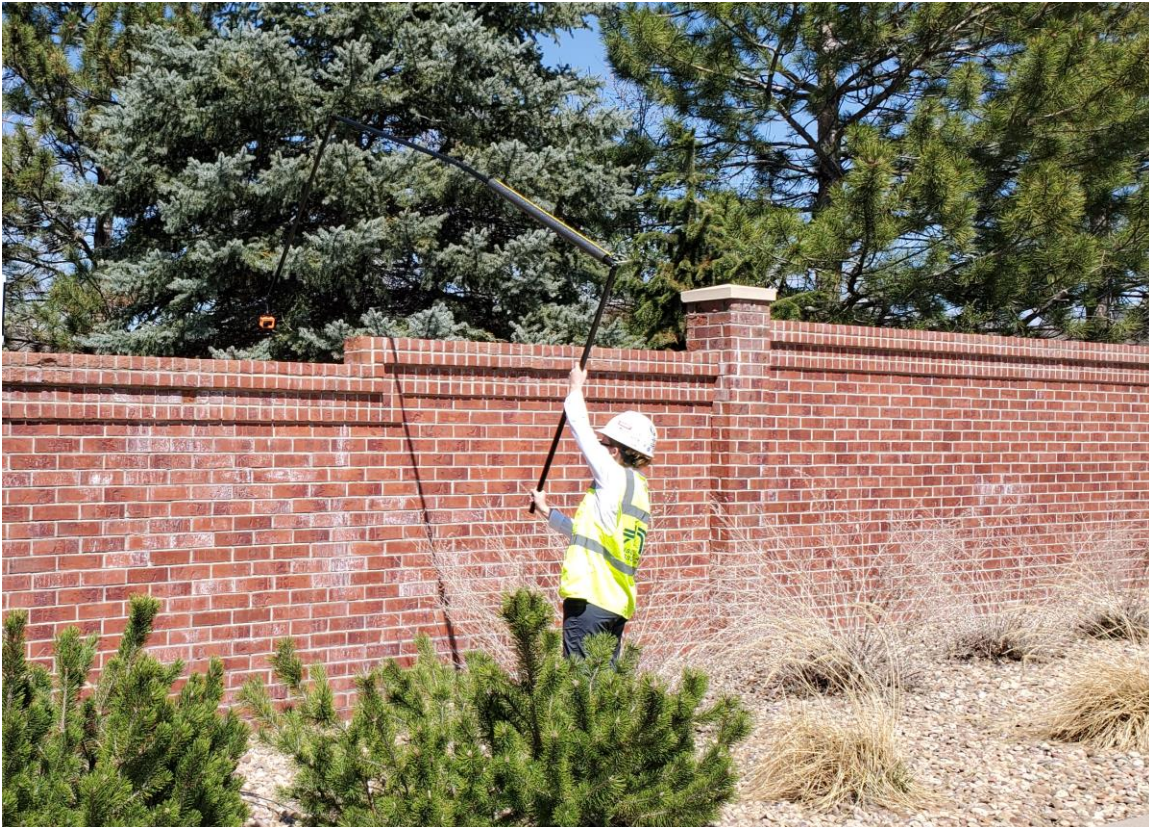
Figure 11. View of camera (with orange protective cover) being lowered over a panel using a boom for photography of the yard side of a panel.
