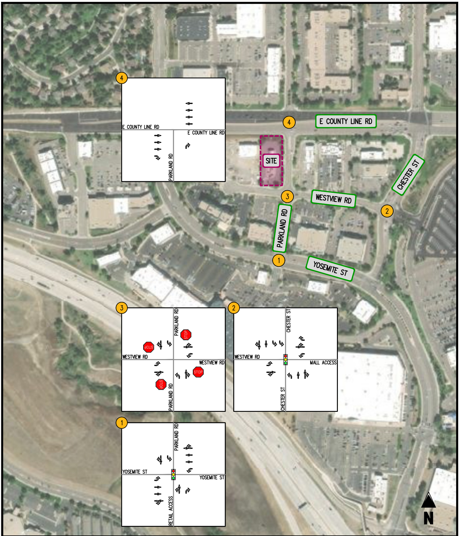
FIGURE 2-1 EXISTING LANE USE AND TRAFFIC CONTROL
